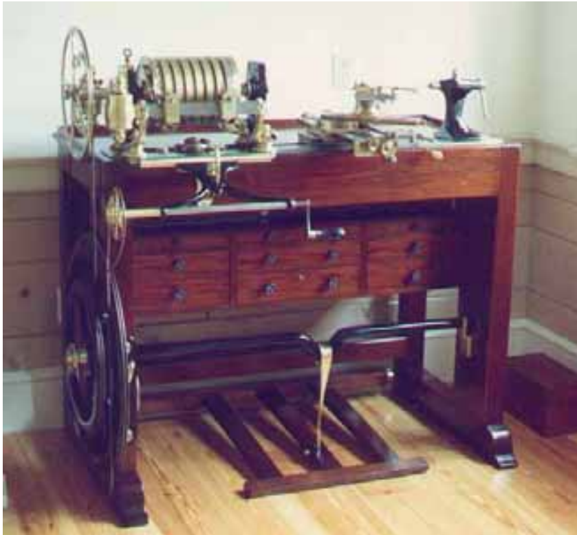
One of the few full Rose Engine lathes made by Holtzapffel
