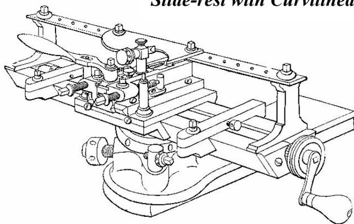
**The Curvilinear apparatus** is for profile copying. It comprises a pair of standards on which is mounted a template bar. The tool-slide guide screw is released and the slide is advanced and retracted by the hand-lever under the control of an adjustable follower or rubber which rubs along the profile of the template. The follower is
