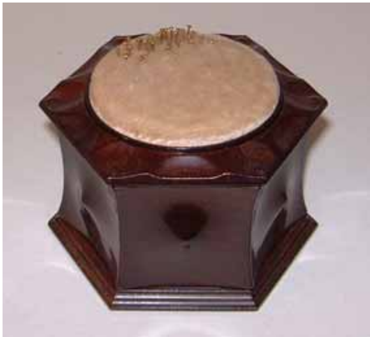
This pincushion box was made on the Dome Chuck; each face was cut with a long round-nosed cutter at maximum radius in the Horizontal Cutting Frame while the chuck was rotated very slowly under control of the tangent screw. The Dome Chuck was counter-balanced to avoid the chuck coming unscrewed or the surface being marred by backlash. The visible crack was caused by leaving this box on the windowsill in bright sunlight!
